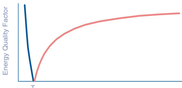
Figure 2. The energy quality factor of heat in relation to the temperature.
