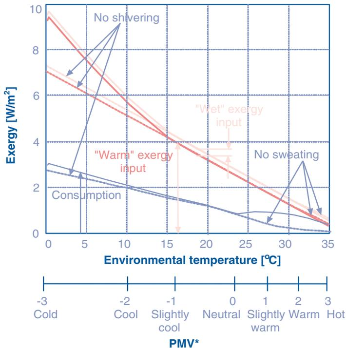
Figure 2. Exergy input and exergy consumption within human body (Watt per unit body-surface area,  $W/m^2$ ) versus environmental temperature ( $^{\circ}C$ ).
