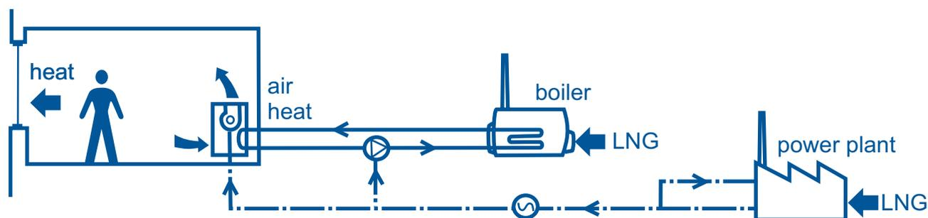
Figure 1. A space heating system assumed for example calculation of exergy consumption.
