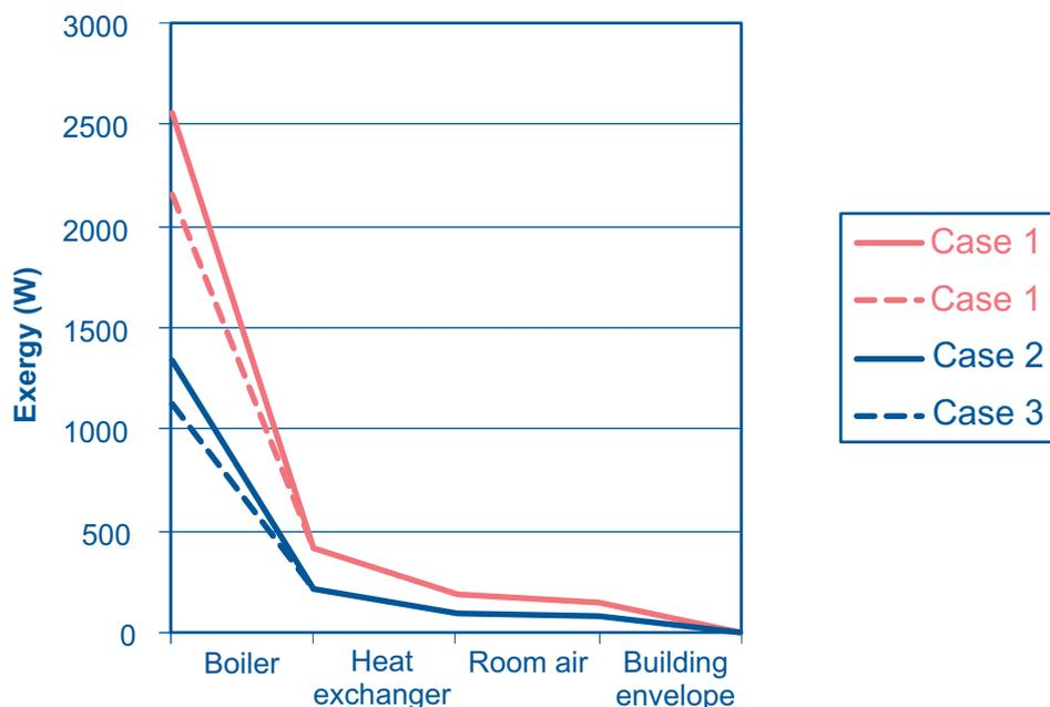
Figure 2. A comparison of exergy consumption for four stages of the space heating systems. Exergy consumption is the difference in exergy between input and output; for example, in Case 1, 2554 W of exergy is supplied to the boiler and 420 W of “warm” exergy is produced and delivered to the heat exchanger by hot water circulation so that their difference, namely 2134 W (=2554-420), is consumed inside the boiler.
