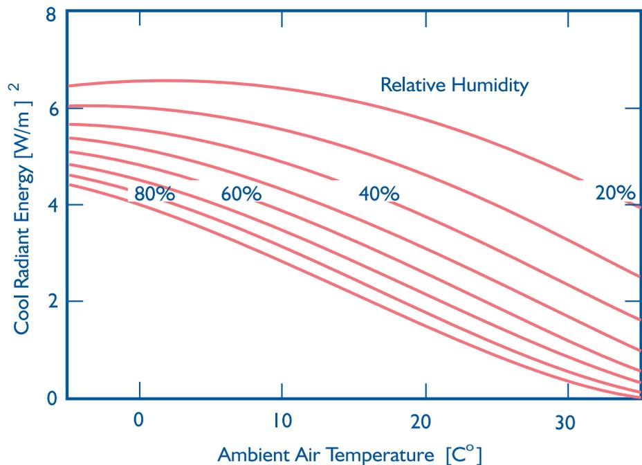
Figure 1. Cool radiant exergy available from the sky as a function of ambient air temperature and relative humidity (Shukuya, 1994).
